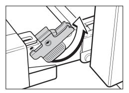
To release the locking clamps on the hinges turn them upwards as far as they will go until they are at an angle. See illustration. Do not attempt to take the door off the hinge guides when it is in a horizontal position. The guides will close, and damage the appliance. Danger of injury.
